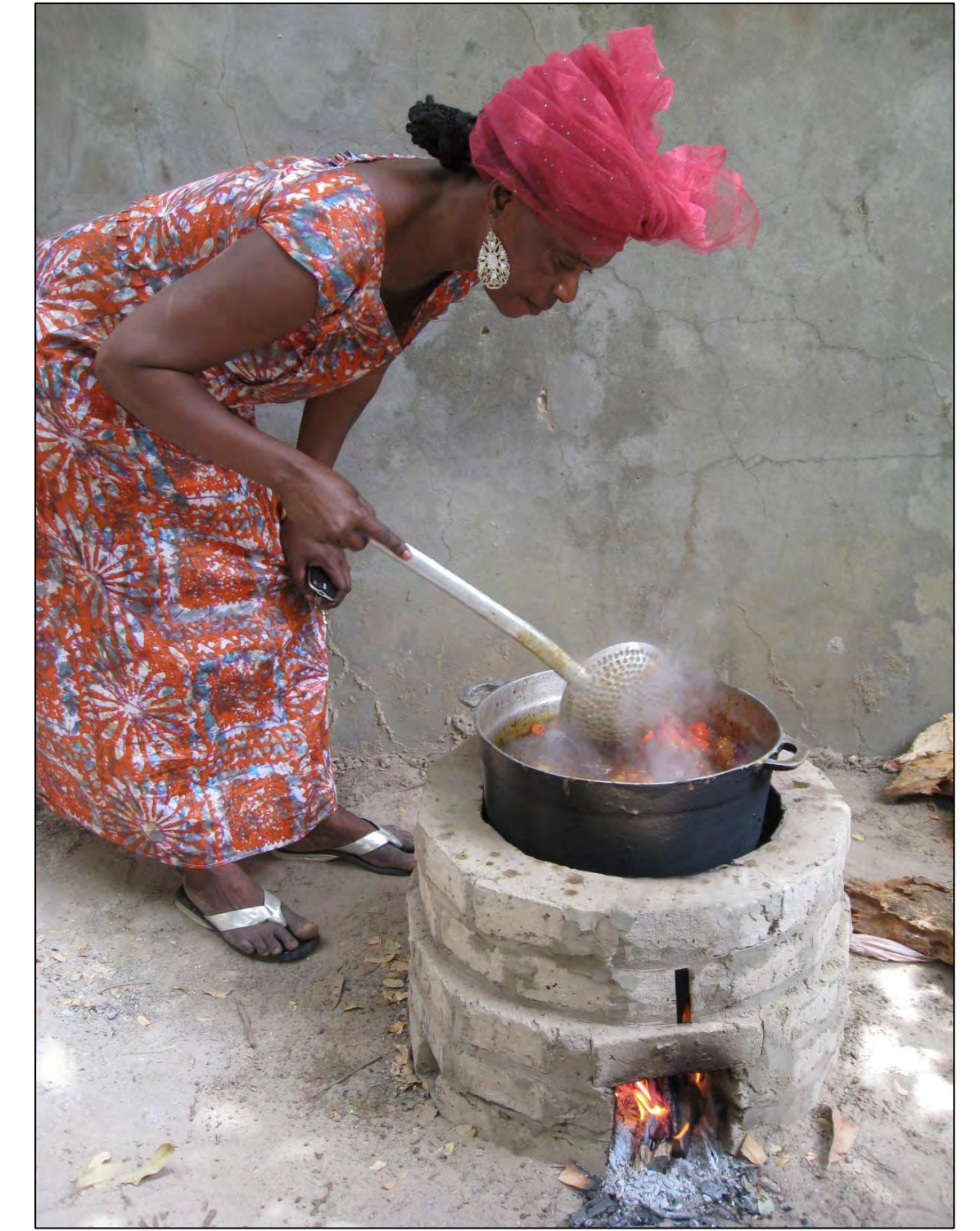
A rural Gambian woman cooking outdoors and breathing easy with the REAP Clay Brick Stove
